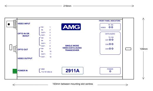
The AMG2911A transmits a single video signal over a singlemode optical fibre. It also transmits two contact closure signals over the same fibre. It is designed to operate with an AMG2912A or an AMG2912AR Video Receiver.
